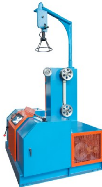
涨立式工字轮放线机 Vertical spool pay-off machine
